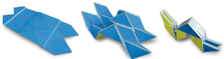
and his colleagues developed a method of assembling thick materials so that the hinges where they meet move in a limited number of ways. The researchers showed how carefully choosing the placement of the hinges and creases allows the structures to move and fold (pictured) in identical ways to origami patterns that use 2D materials.
